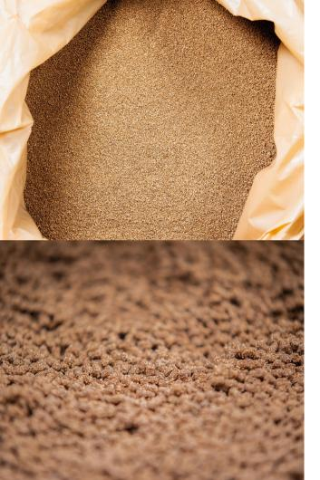
Sughera® is a **REVOLUTIONARY** material consisting of synthetic rubber blended with micro granules of natural cork. For the first time, micro-agglomerated natural cork pieces are molded by injection and shaped without using any glue.
